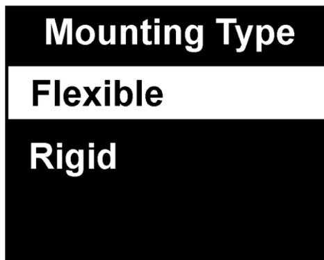
As a basic “rule of thumb”, unless a machine is bolted down to a concrete floor, its mounting should be considered as being **flexible**.
