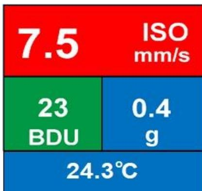
Taking a reading causes the overall vibration numbers and temperature screen to be displayed as shown in the example screen left. Note: Temperature will not display if a standard low power accelerometer without temperature (p/n A9100) is used.
